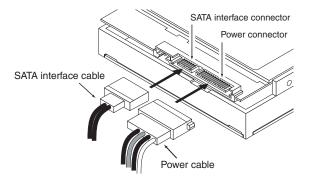
Figure 2. Attaching SATA cabling
